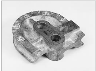
Fig. S30 — Radius Block for use with HB632 Bender
